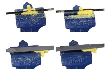
The modified brake blocks for 2-piston calipers should look like the pictures at the right.
