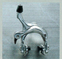
Low friction designed Dual-Pivot Brake
